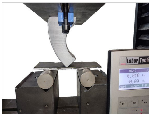
Figure 1: A 3D-printed PLA V-bending die under load in a universal testing machine — one of six sheet grades used to map the die's real destructive limit.
