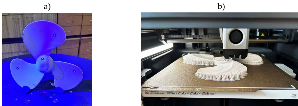
Figure 1. a) 3-blade propeller during scanning, b) 3-blade propeller model during printing
