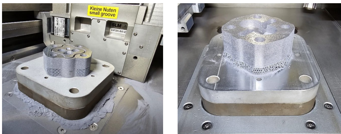
Figure 1. Manufactured hydraulic pump body with internal noise-reducing structure.
