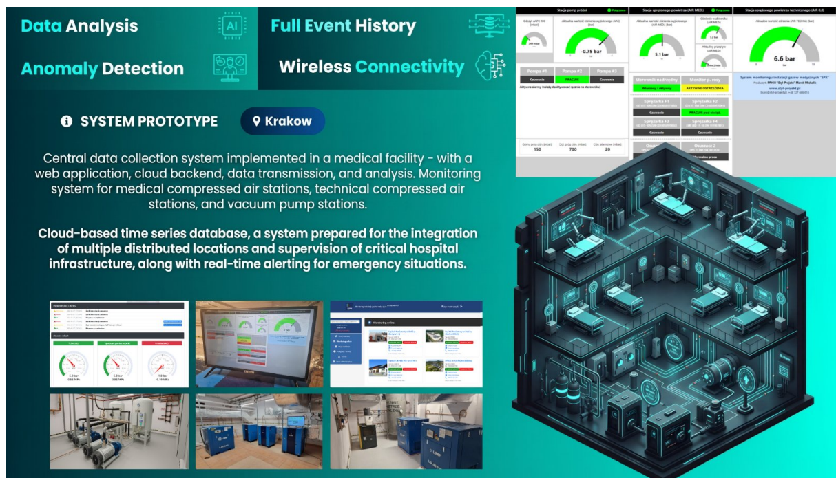
Figure 1. A cloud-based distributed intelligent monitoring system for medical gas pressures
