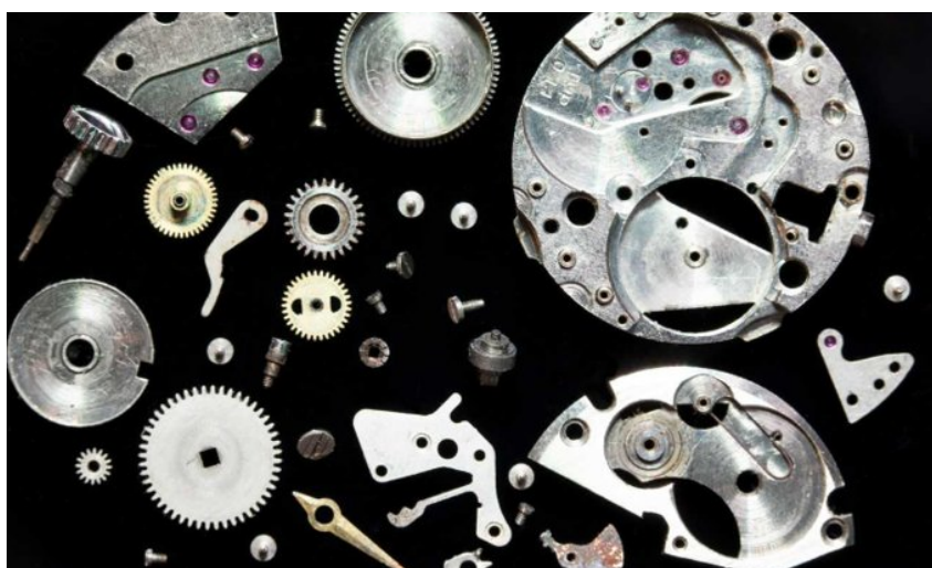
Figure 1: Overall picture of disassembled components of calibre K25
