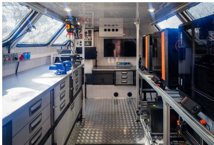
Figure 1. Interior of the MAMS, showing the post-processing area (left), the additive manufacturing area (right), and the CAD/CAM and 3D scanning area (centre)
