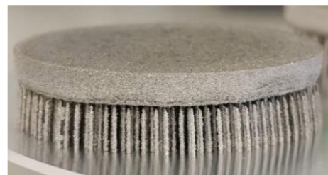
Figure 5. 3D-printed discs for mechanical testing
