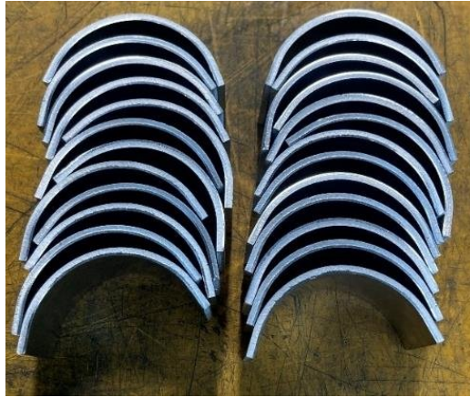
Figure 2: The same rapid-tooling approach at production scale: 275 aluminium stabilizer-clamp inserts formed by a 3D-printed PLA die, at roughly 3% of the material cost of a machined steel tool.
